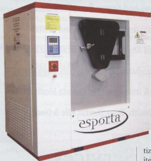
An Esporta unit removes dirt with high-pressure hydraulic action.
